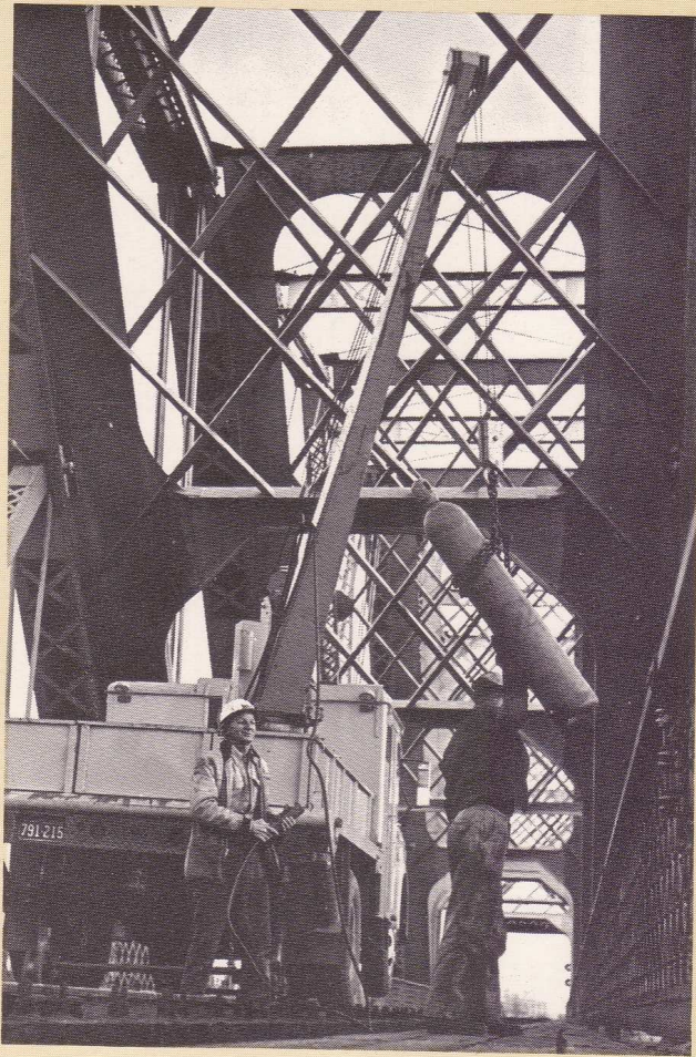
Truck equipped with flanged wheel attachments which permit its operation over rails as well as highways.
