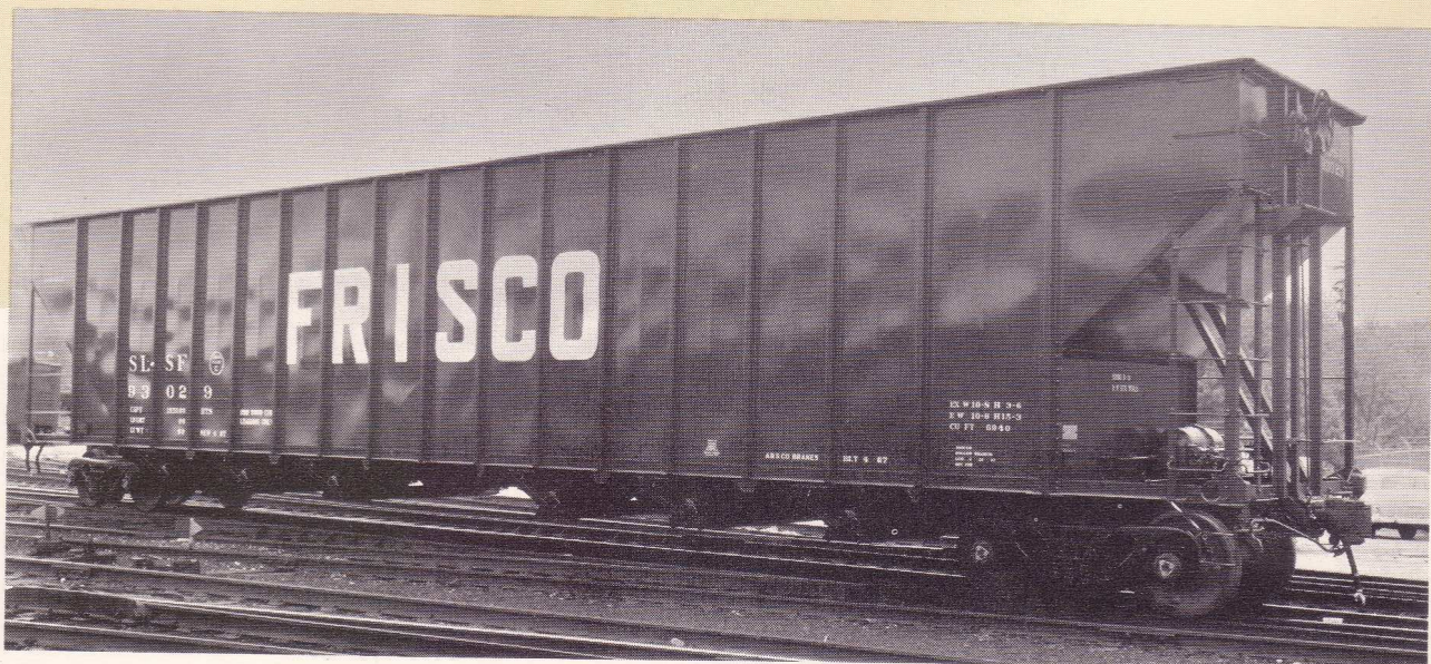
Jumbo open top hopper car. With a capacity of 7,000 cubic feet, these 100-ton cars are used primarily for transporting wood chips for forest and paper product patrons.
