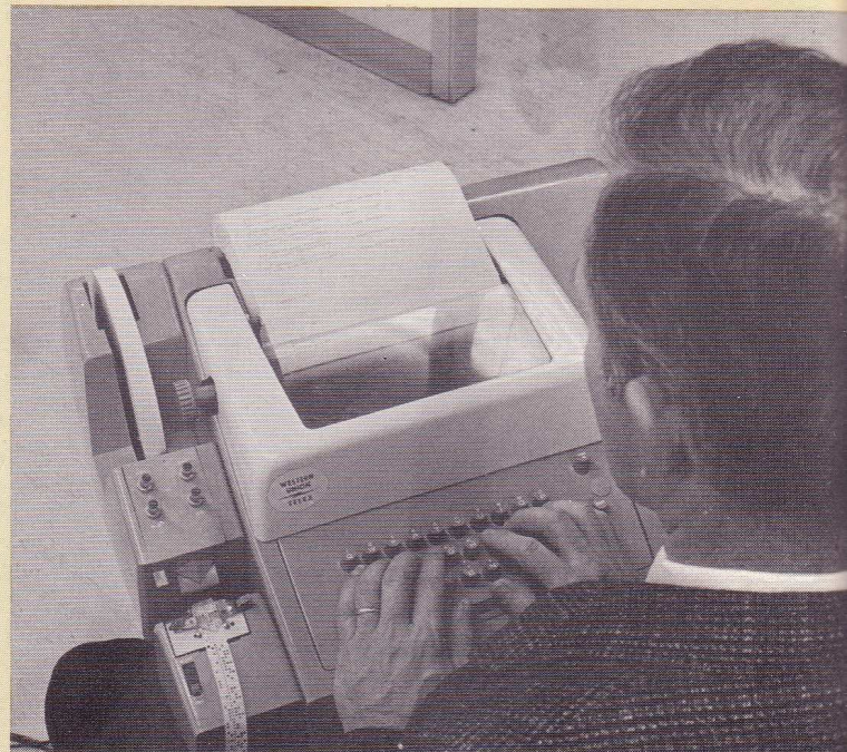
Through the use of this Telex machine, some 40 Frisco off-line traffic offices have instantaneous communication with the Company's computer at Springfield, Missouri, thus making it possible to supply patrons with up-to-the-minute information on their shipments.
