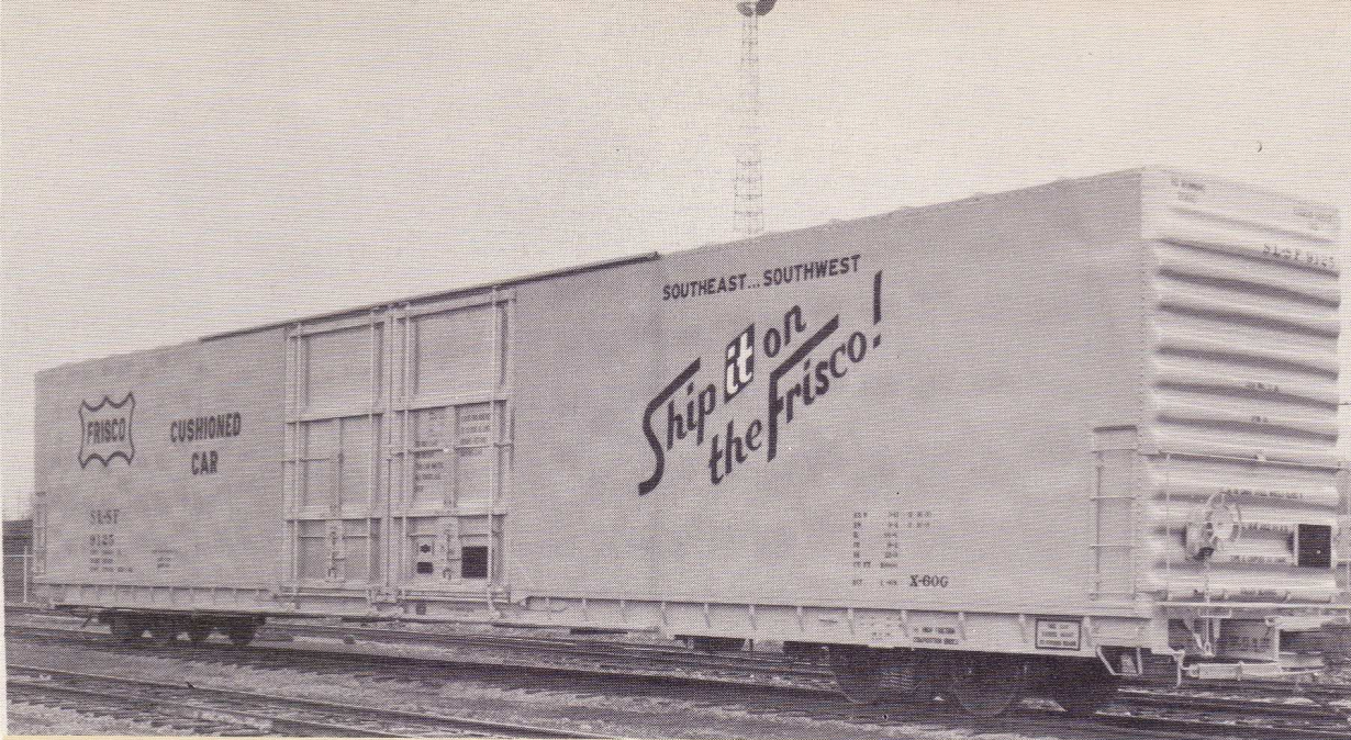
High capacity, cushioned underframe box car used exclusively for hauling automotive parts. Frisco owns 34 of these. Each car costs about $30,000 exclusive of interior devices.
