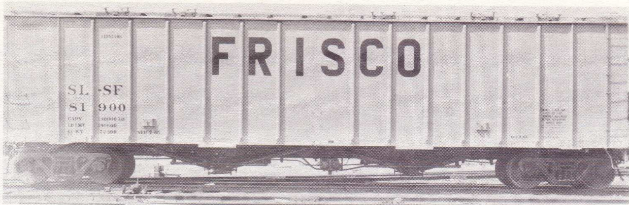
Airslide car with roller bearings. Capacity: 4,180 cubic feet — 100 tons.
