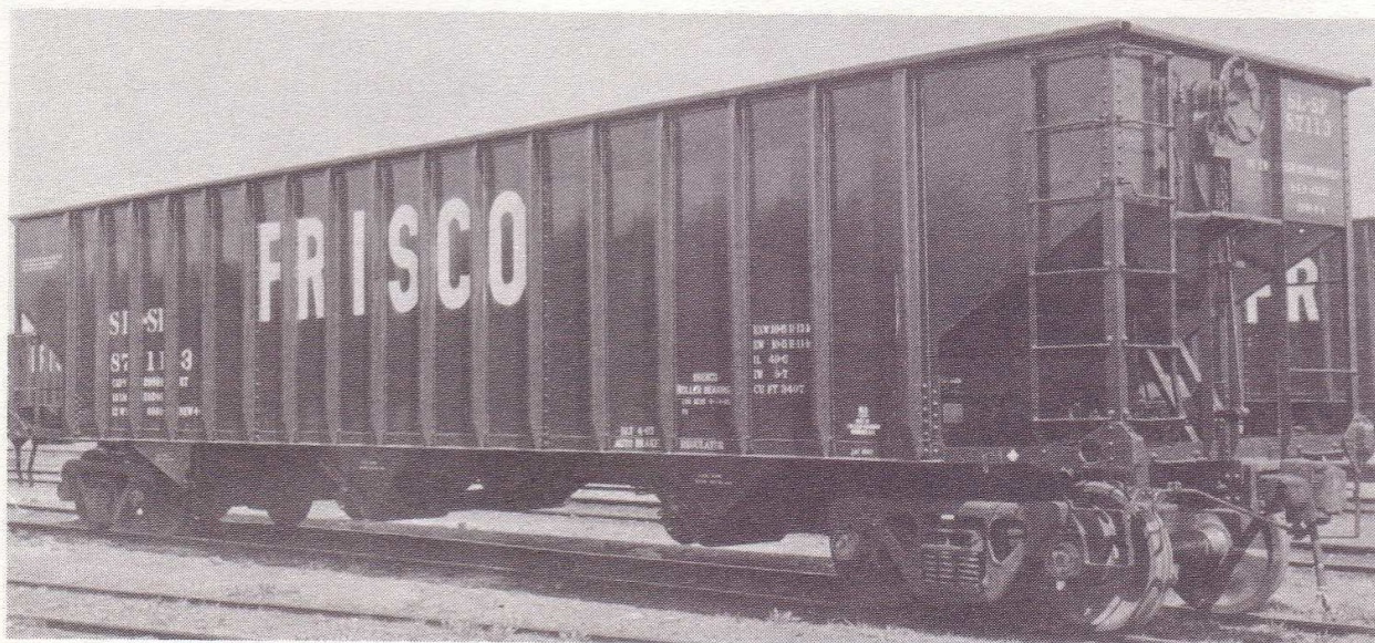
Open top hopper car with roller bearings. Capacity: 100 tons.
